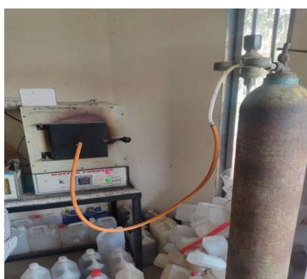
Muffle Furnace with Nitrogen Cylinder
